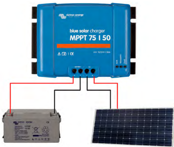
Figure 1: Power connections
